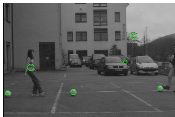
Fig. 4.1: Situation with three balls and structured background. Potential balls found by the evaluation of the Hough accumulator are marked.
