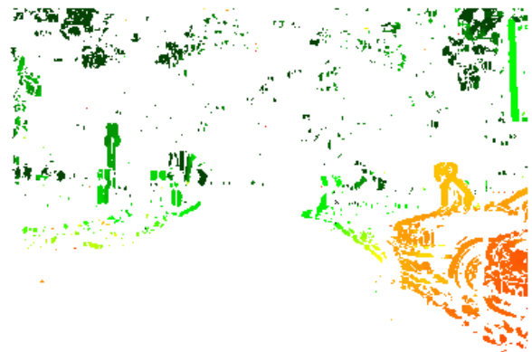
Fig. 2.1: Color encoded disparity image generated by the correlation approach. Red signals close, green means far.
