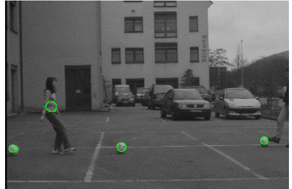
Fig. 4.3: Remaining ball candidates after size and position check.
